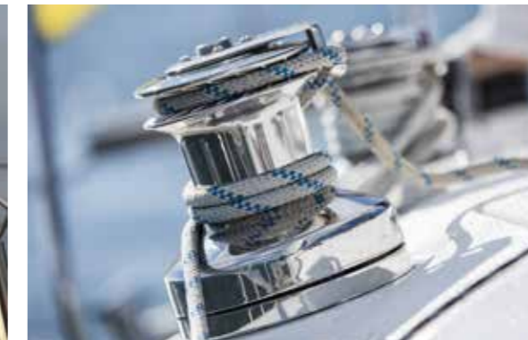
Andersen full stainless steel self-tailing winches are standard on all Najad models.
