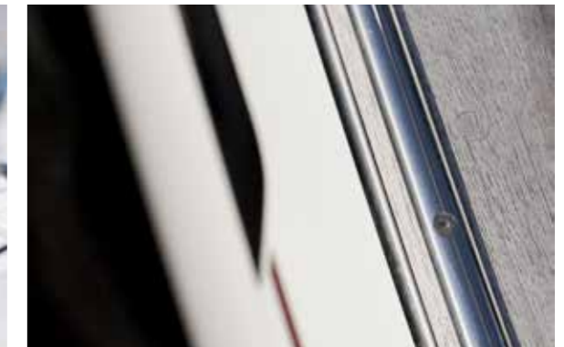
Teak capping fitted with stainless steel rail on the outside for best possible protection.
