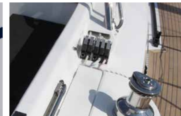
Clean and safe with halyard lead under deck to cockpit jammers and winches.
